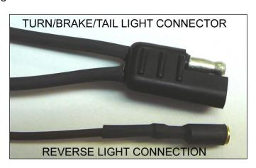
➤ Using the pre-installed socket terminal, the Black/Red wire tagged "Reverse" will plug into the molded male connector.
