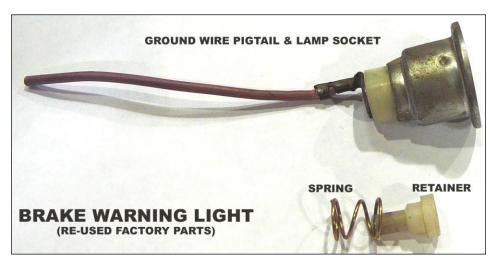
In order to make the proper connections to the BRAKE WARNING LIGHT, the factory lamp socket, spring, and retainer must be re-used.
