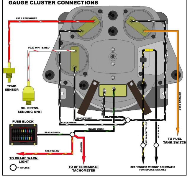
. **NOTE:** If the Ammeter reads backwards after installation, you have the wrong wire running through the loop. Disconnect the 2 wires and run the Black/Yellow wire through the loop on the GAUGE CLUSTER.
