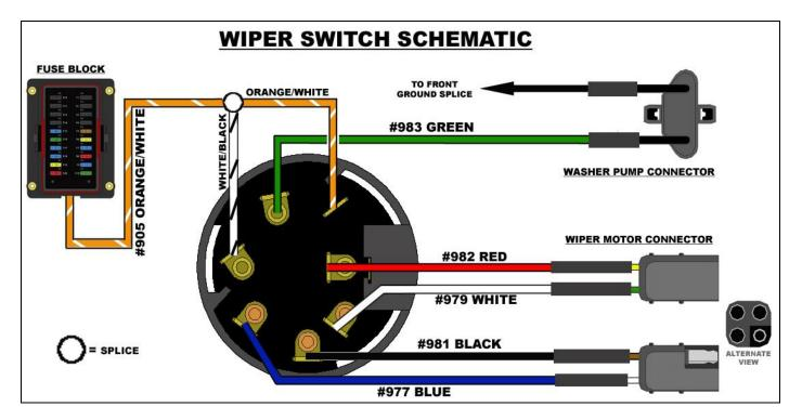
For those with a 1966 or 1967 Bronco with vacuum wipers and a WASHER BUTTON on the dash, only 2 wires from the WIPER SWITCH portion of the Painless harness will be used; the 2 longer wires.
