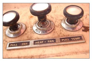
In 1973 Ford started installing label indicators between the Switches and under the Climate Controls on the dash. These labels can be seen in the picture to the left and on the 1973-1977 DASH LAYOUT drawing on page 24. If you have a 1966-1972 dash, you can skip this step and move on to the next connection, the Gauge Cluster.
