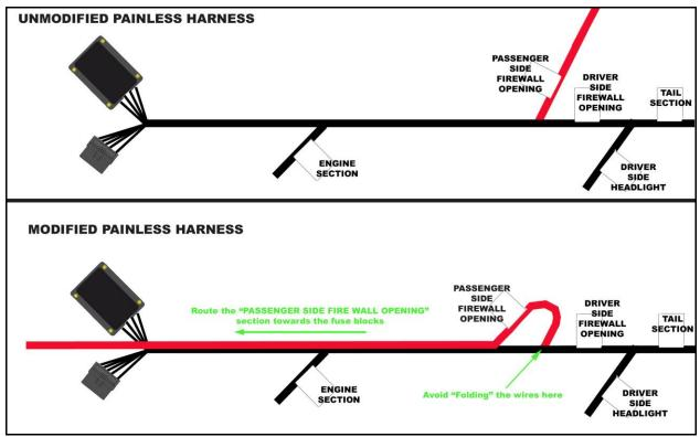
**PAINLESS HARNESS MODIFICATION**: this drawing does not show individual wires, only sections Also, this modification only needs to be done by those with a passenger side firewall hole.
