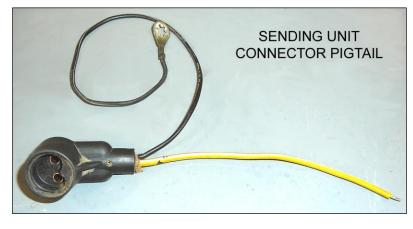
the Black ground wire. This ground wire will be re-used in order to re-connect the ground to its factory location.
