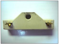
The Ballast resistor, seen in the photo to the left as well as in the following drawings, is supplied in the bag kit that accompanied the Painless harness. This Ballast Resistor replaces the factory resistance wire between the COIL and the Ignition Switch. If you have an internally resisted COIL or using an MSD Ignition box, the resistor will be omitted. If you do not have either of these, the Ballast Resistor MUST be used.
