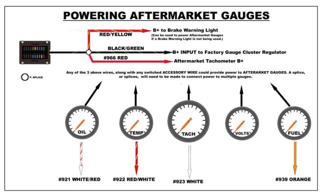
On applications where AFTERMARKET GAUGES are replacing the factory Gauge Cluster or a factory Gauge, the sender wires from the Painless harness will work with the new gauge just as it did with the factory gauge. These sensor wires can be seen on the **POWERING AFTERMARKET GAUGES** drawing on the previous page or on the **WIRING AFTERMARKET GAUGE** drawing below.
