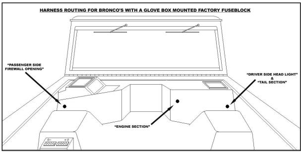
FACTORY FIREWALL HOLES: Sections listed are routed through the holes they are pointing to
