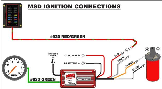
Consult the manual that came with your MSD Ignition box for information and diagrams concerning connection of the White wire or the Magnetic pickup.
