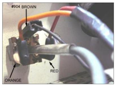
Heater switch connection requires 3 wires:
