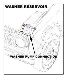
The WASHER PUMP connection offered in the Painless harness has a connector installed. This connector will only fit the pumps used on the factory Electric Wiper vehicles. The 1966-1967 vehicles will have a different style WASHER PUMP unless they have been retro fitted with the later style PUMP. For those with the early style PUMP, your instructions follow the instructions for those with the electric Wiper System PUMP.
