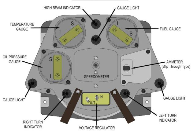
The GAUGE CLUSTER portion of the Painless harness is made up of 2 break outs. All GAUGE CLUSTER wiring will be tagged with their function ("High Beam Indicator", "L. Turn Indicator", "R. Turn Indicator", 3 "Gauge Light"s, "Oil Pressure", "Temperature", "Fuel Gauge", "Ammeter", and 2 wires tagged "Voltage Regulator".
