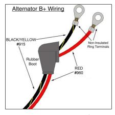
There are many different alternatives pertaining to the charging system and ALTERNATORS used by owners. Red #960 is only necessary on High Amperage Alternators, 65 amps or more. It may be omitted to reduce clutter on the back of the ALTERNATOR if the amperage is 65amps or less. Make the connections to the ALTERNATOR according to the following drawings representing the ALTERNATOR you are using.
