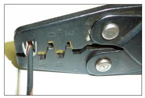
With Strap 1 crimped you can move onto crimping the insulation strap, Strap 2. Place Strap 2 into the appropriate jaw of the crimpers. This jaw will be larger than the one used to crimp the first strap. Crimp down on Strap 2 making sure the strap folds downward into the wire, and not overlapping itself, refer to the drawing
